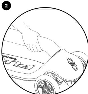
Grip the handlebar so that you fully depress button (1) located at the bottom of the handlebar.
